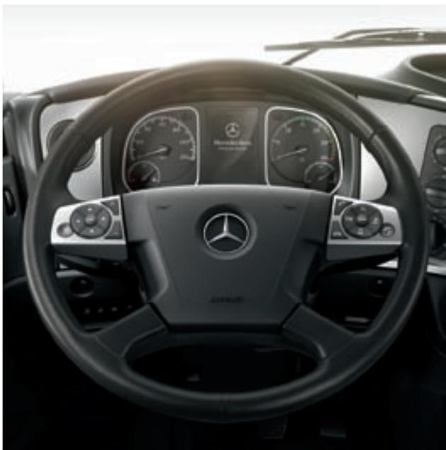
**Multifunction steering wheel.** The standard-fit multifunction steering wheel makes light work of various functions: apart from the radio and telephone, the cruise control can now also be operated via the steering wheel. Many other vehicle functions and diverse settings can also be controlled in the new instrument cluster
