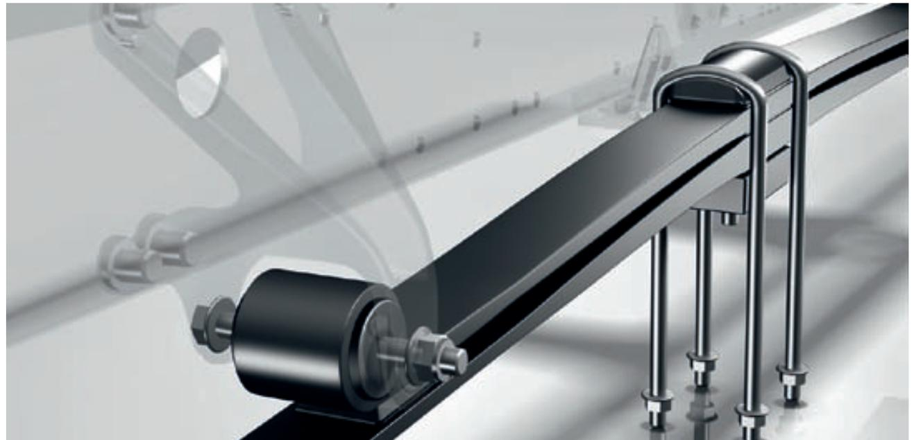
**Steel suspension.** The new Atego comes with weight-optimised multi-leaf parabolic springs for a high standard of ride and suspension comfort both on- and off-road
