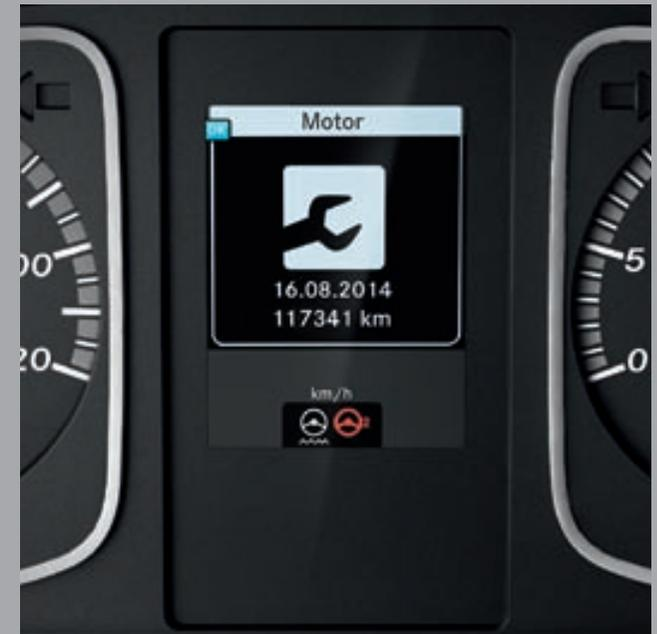
**Dynamic maintenance computer.** The new Atego is equipped with a dynamic maintenance computer. “Dynamic” means that maintenance intervals are now calculated on the basis of actual wear, rather than driven mileage. This enables service products and fluids to be used to the full and maintenance work to be combined in an effective manner
