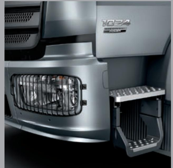
**Geared to operational needs.** The moving entrance step on the Atego all-wheel-drive variants illustrates how the new Atego is geared to specific operational needs. And details such as the optionally available headlamp protection grilles prevent damage while at the same time enabling swift and simple cleaning of the headlamps
