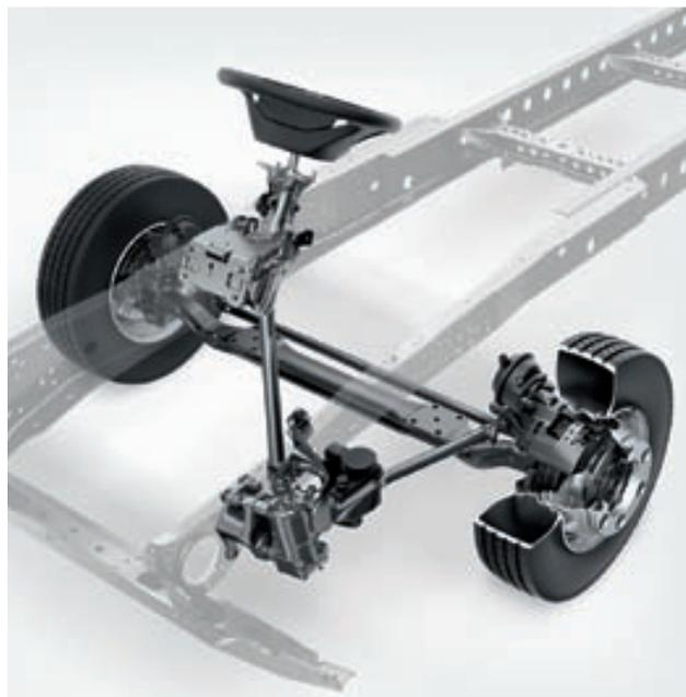
**More precise steering.** The Atego's new steering provides for simple, exact handling during manoeuvring and for reliable straight-line stability and high directional stability at high speeds. A further advantage of the new steering is enhanced steering precision, requiring less corrective action on the part of the driver
