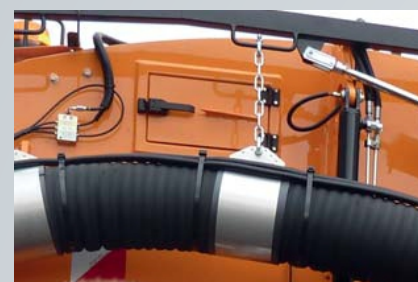
Cleaning hatch for suction channel
