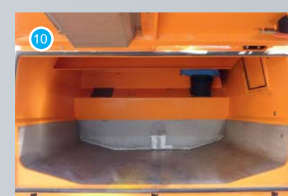
The large debris container
