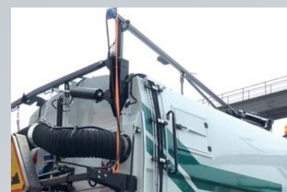
Roof arm for high-pressure lance
