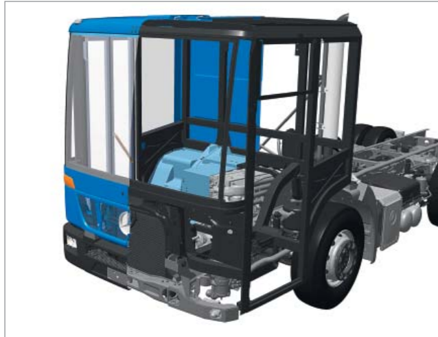
Aluminium space-cage cab: the Econic cabs have a lightweight aluminium space-cage structure and meet the requirements of the European ECE R29/2 crash-test standard
