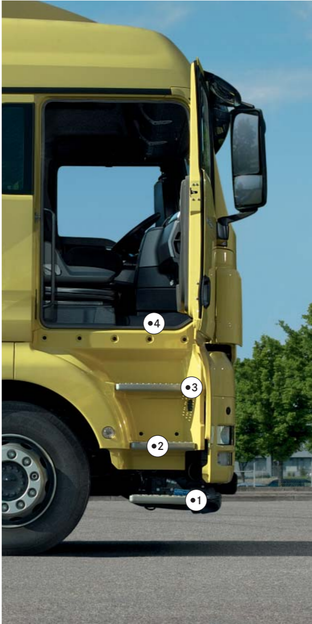
Conventional cab: entering a conventional cab involves a climb. Steps of differing heights (1–4) increase the time required to perform work processes
