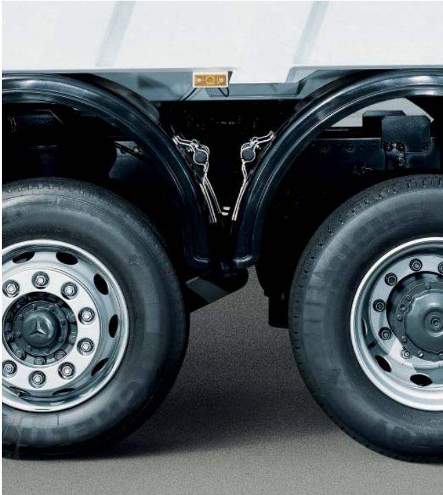
Raising/lowering function: depending on the variant and application, the raising/lowering function allows the Econic to be raised by up to 200 mm and lowered by as much as 60 mm
