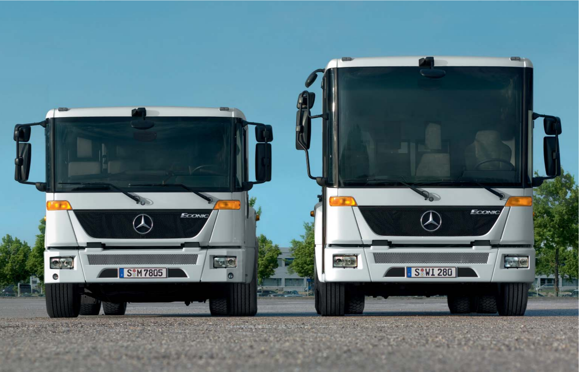
Cab variants: the low cab allows the use of higher bodies while the high cab offers more comfort
