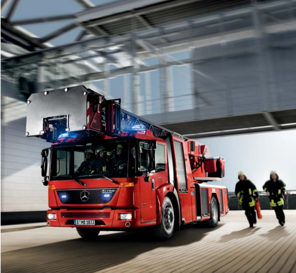
Econic turntable ladder vehicle: with an overall height of just three metres, it can reach the scene of the emergency quickly and directly without having to avoid low underpasses
