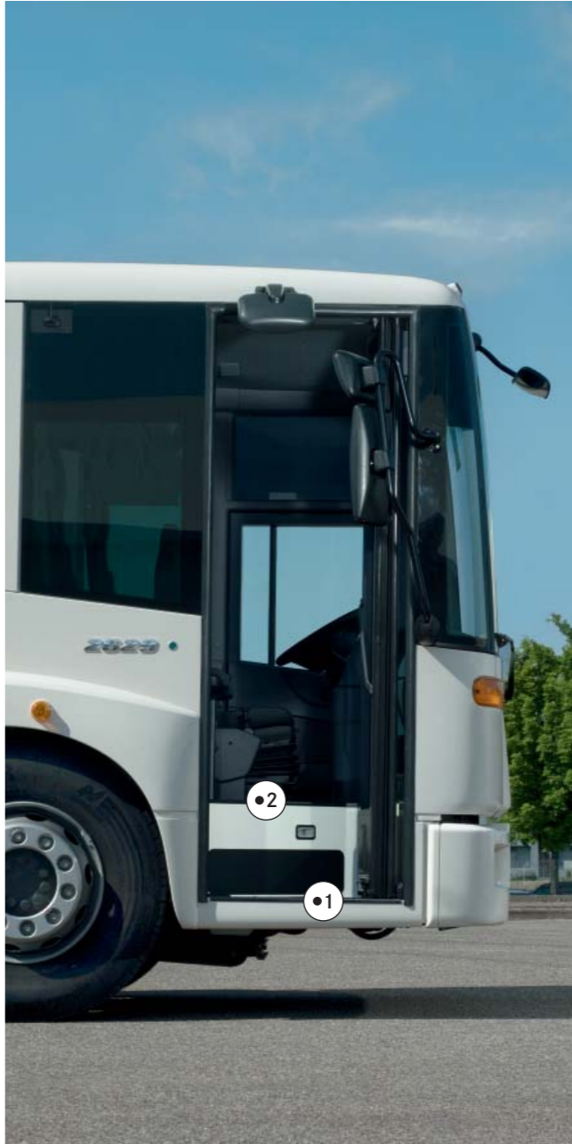
Econic low-entry design: boarding the Econic involves only one (1–2) step – protected by its integrated position in the cab, it has a rugged surface for optimum grip and fast boarding/alighting
