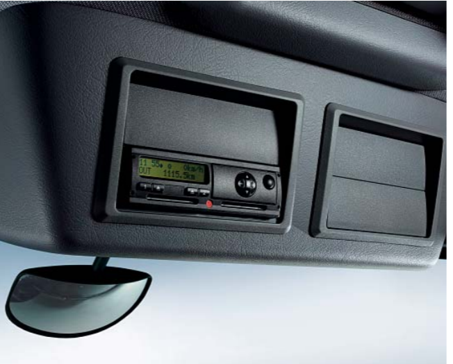
Pre-installation for communications equipment: four DIN slots in the area above the windscreen provide a secure, easily accessible installation space for the tachograph, Toll Collect unit or FleetBoard unit
