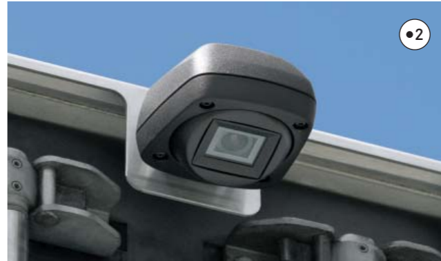
A better view: optimum visibility is ensured by the modified mirror array (1) with the upper wide-angle mirror and, below it, the main mirror, as well as by the optional reversing camera (2). The one-piece sunblind (3) offers effective dazzle protection even when the sun is low in the sky
