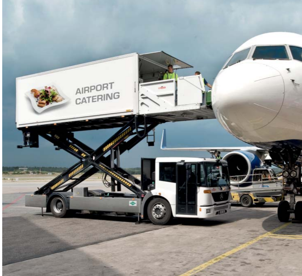
Econic Catering vehicle: with scissor lift the Econic can easily supply all types of aircraft
