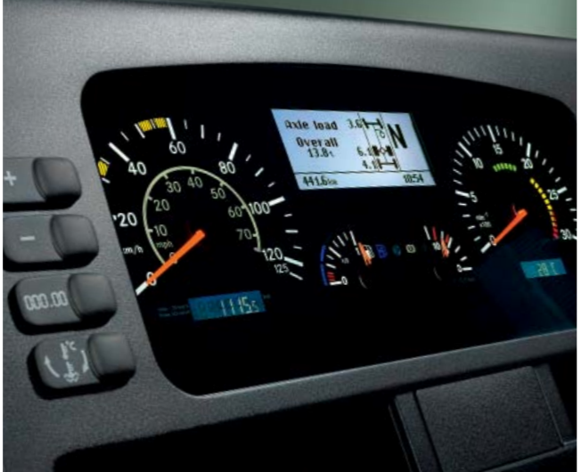
Instrument panel: the central axle-load measuring system provides a continuous display of the current load status and the gross weight of the individual axles
