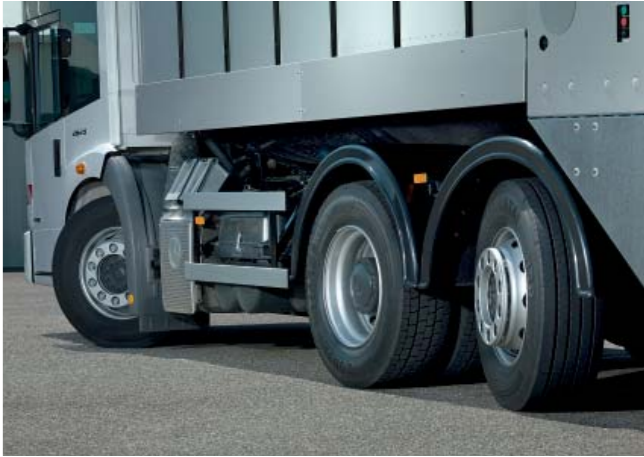
Forward-trailing or trailing axle: the optional electro-hydraulically steered forward-trailing or trailing axle makes the Econic extremely manoeuvrable
