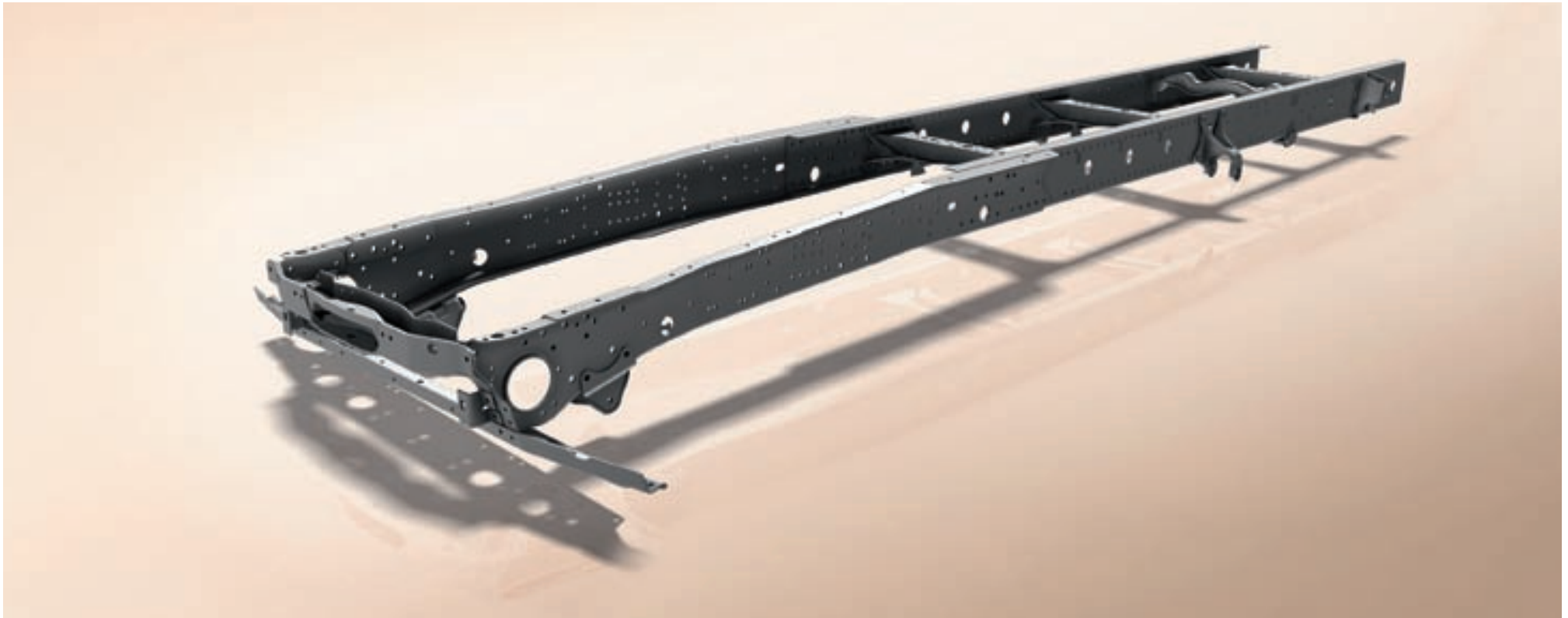
The Atego's frame was developed specifically for urban distribution. It combines low weight with a highly robust design, while its 'Z' shape and a dense hole pattern make for good body-mounting ability. What's more, it enables a very low entrance height and convenient access through to the co-driver's side
