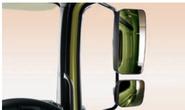
Ample dimensioned exterior mirrors with a manual heating control maintain an optimum all-round view at all times in urban and regional distribution. The wide-angle exterior mirror is attached at the bottom for a better overview and reduces the blind spot still further
