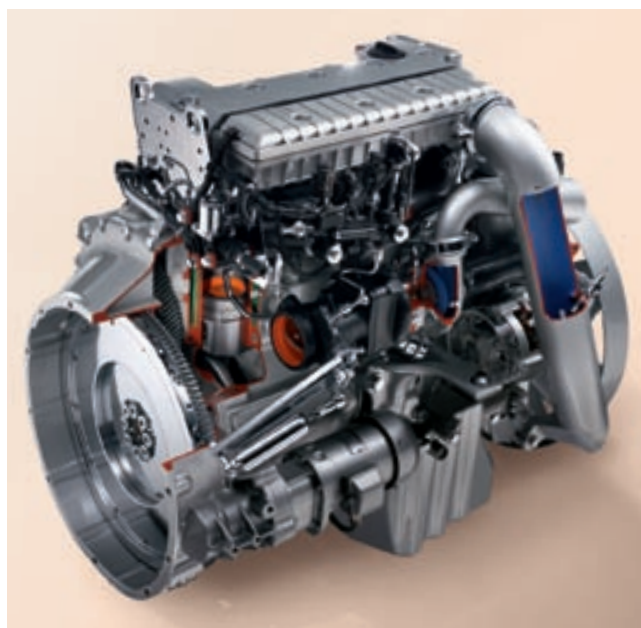
The 4-cylinder in-line engine with a displacement of 4.8l and an output of 160 kW (218 hp) delivers the sort of performance usually associated with six cylinders. A further benefit of this powerpack is that it weighs a good 100 kg less than a 6-cylinder engine with comparable performance
