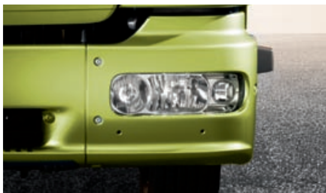
Not only do the clear-lens headlamps on the Atego look good, they ensure optimum visibility and safety for urban distribution. The monochrome indicators are integrated into the radiator grille
