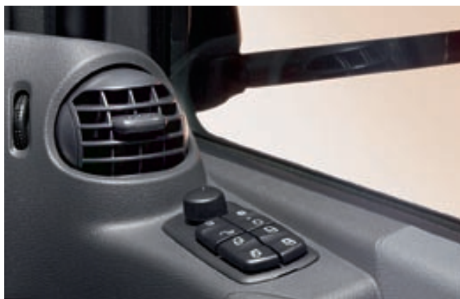
The door control panel groups together important switches, such as those for operating the electric windows, the mirror adjustment and the mirror heating. The eyeball vent boosts both safety and comfort by preventing the side windows from misting up in winter
