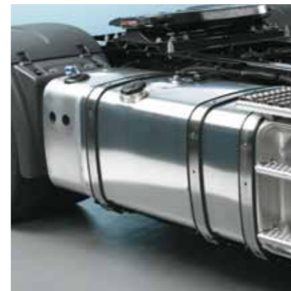
Combination tank for diesel and AdBlue®.
