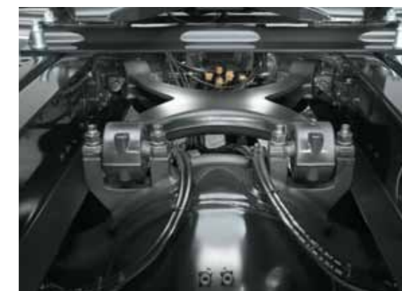
Weight-optimized X control arm with stabilizer and control arm function for semitrailer tractors and high-load roll stabilization for 6x2 vehicles.
