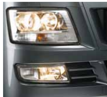
Headlights with free-form reflectors, Xenon dipped headlight.
