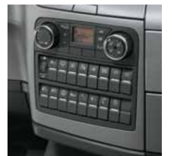
Controls for the air-conditioner, heater and ventilation. Switch field with function displays.
