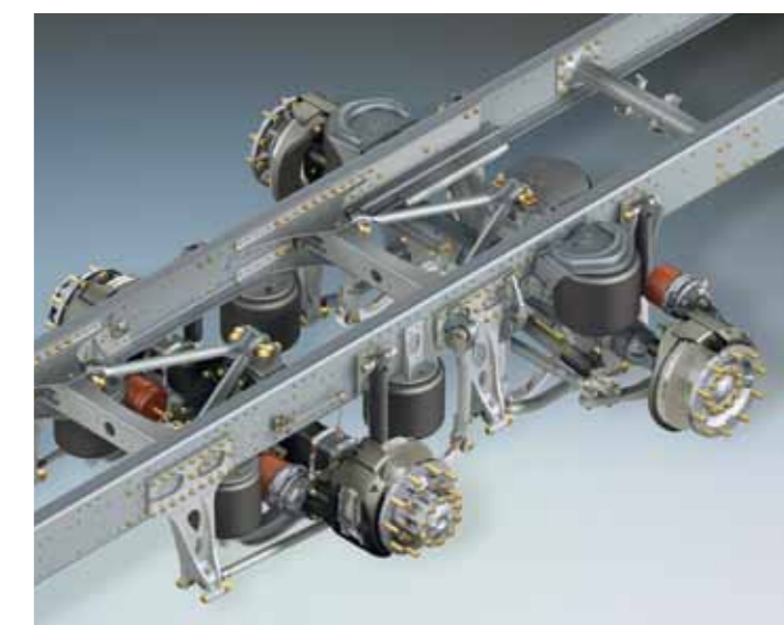
Steered trailing axle with air suspension for the TGM.
