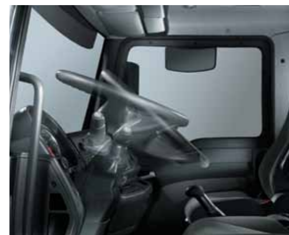
Button in footwell for stepless adjustment of steering-wheel height and angle.
