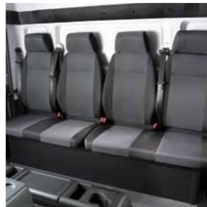
Second row of seats in crew cab, all seats with three-point belts.
