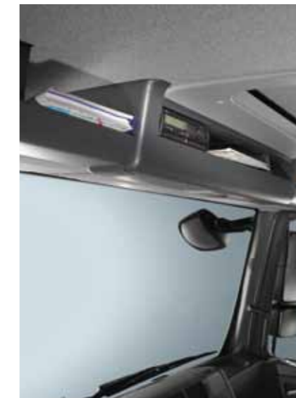
Storage compartment above windscreen and roof skylight in C cab.
