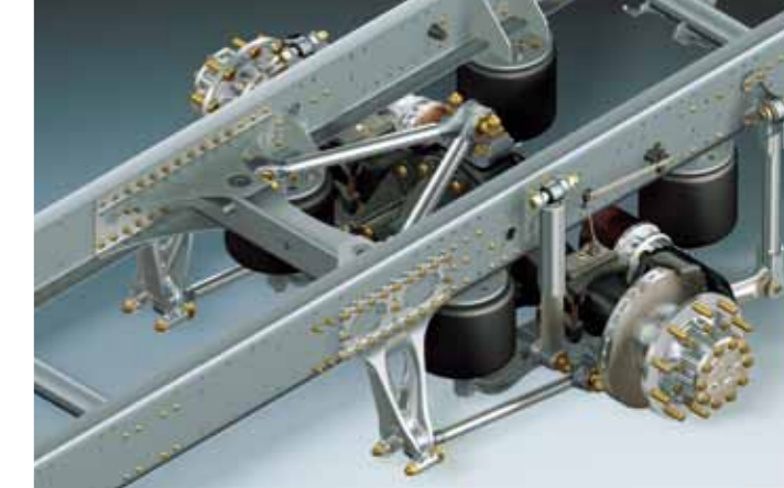
4-bellows rear-axle air suspension for the TGM. Optional heavy-duty rear axle, load capacity 11.5 tonnes.
